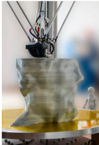
torso while being printed with a delta-printer
