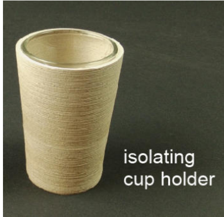
thermal isolating because of pores low thermal conductivity
